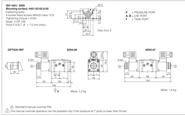
Overall dimensions refer to valves with connectors type 666
